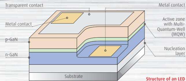
**Did you know ... ?** The scientific explanation of how an LED works: An LED has an active zone that determines the color of the light. This is embedded in a p-doped layer and an n-doped layer that transport electrons (n-doped side) and so-called "holes" (p-doped side) to the active layer when current is flowing.
