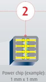
After the **deposition process**, the wafers are processed into chips, finally resulting in the production of a finished LED. Depending on the chip size, a 4 inch wafer can deliver between 4,000 and 120,000 LED chips.
