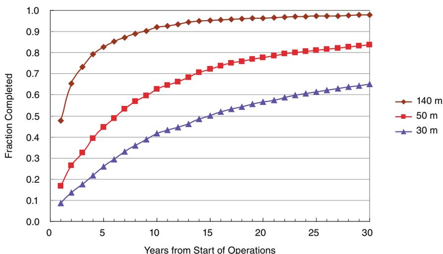
**FIGURE 3.9** Years to completion for a shared Large Synoptic Survey Telescope (LSST) for near-Earth objects (NEOs) with diameters greater than or equal to 30, 50, and 140 meters. The shared LSST achieves 90 percent completion of the survey for potentially hazardous 140-meter-or-greater-diameter NEOs within 10 years of start of operations. SOURCE: Courtesy of Steve Chesley, Jet Propulsion Laboratory.
