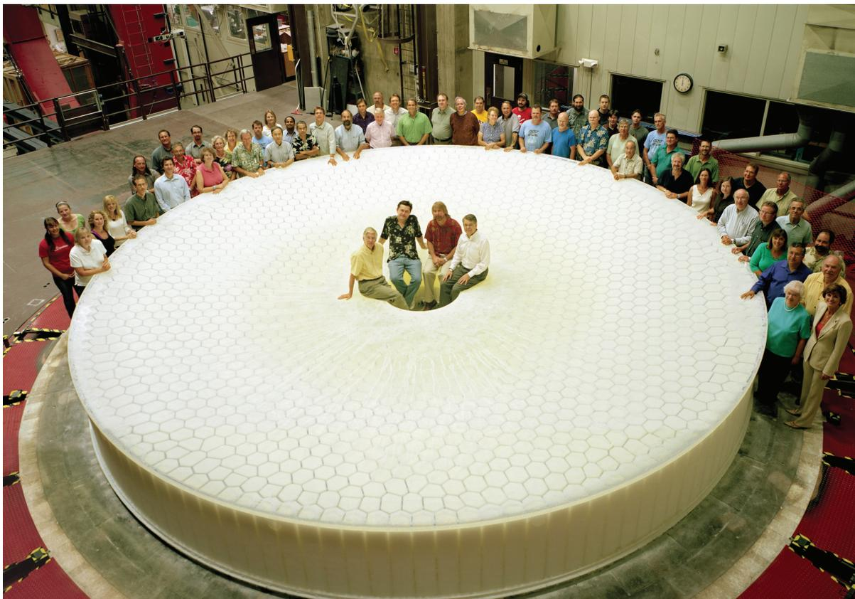
**FIGURE 3.1** The Large Synoptic Survey Telescope 8.4-meter-diameter mirror after being successfully cast at the University of Arizona Mirror Laboratory. SOURCE: Courtesy of Howard Lester, LSST Corporation.
