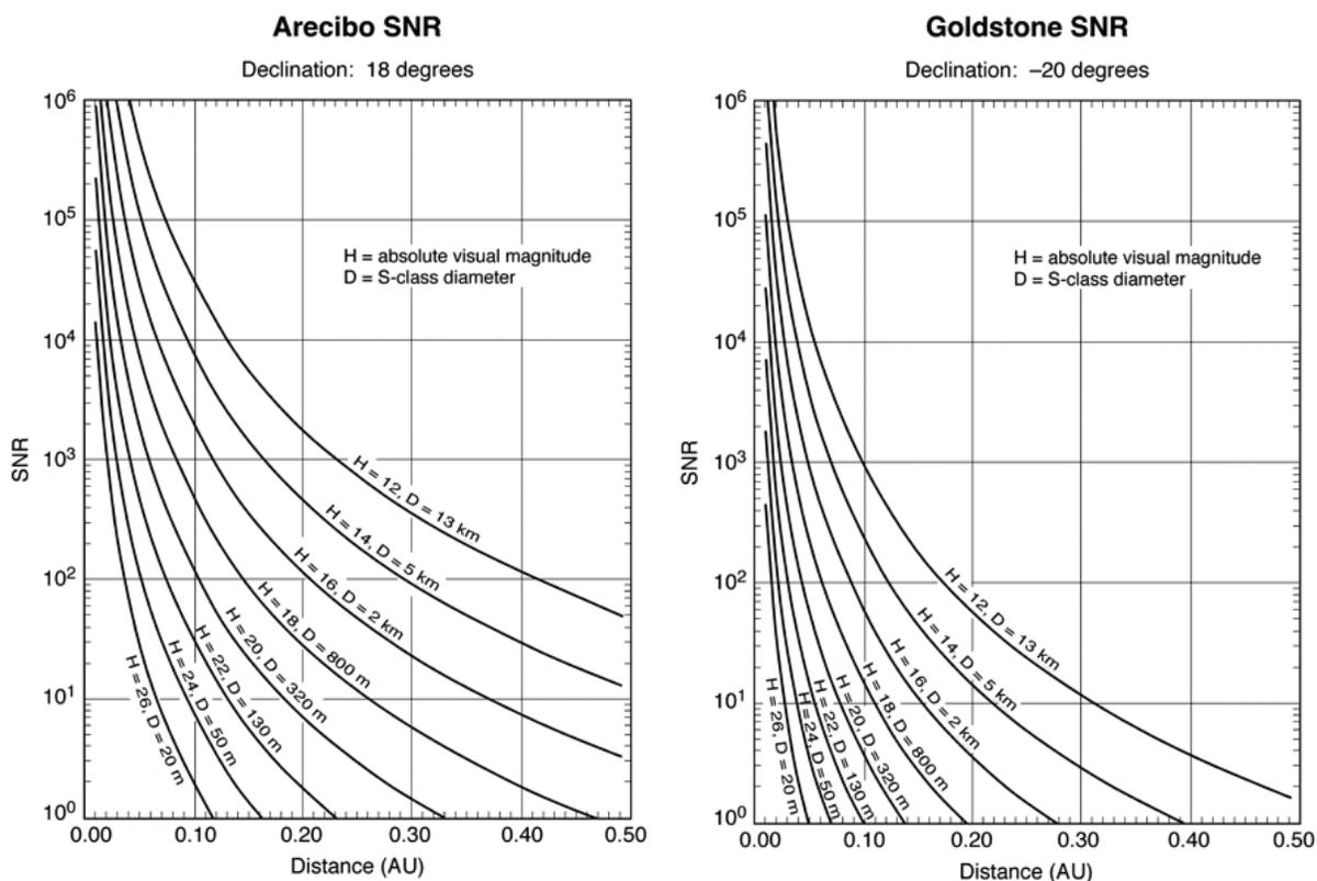
**FIGURE 4.4** Signal-to-noise ratios (SNRs) for radar echoes received at the Arecibo Observatory and Goldstone Solar System Radar for several combinations of distances and sizes. “S-class” is a category of stony asteroids. SOURCE: Courtesy of Lance A.M. Benner, NASA, JPL.
