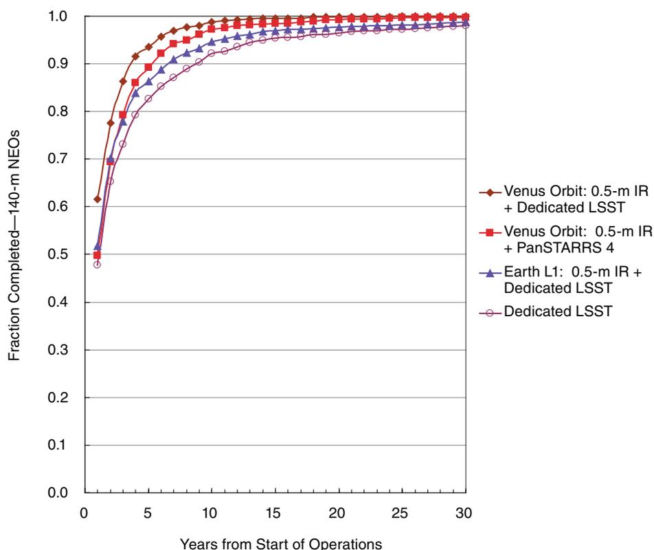
**FIGURE 3.8** Years to 90 percent completion of the congressionally mandated survey for the detection of potentially hazardous near-Earth objects (NEOs) 140 meters in diameter or larger for combinations of space-based 0.5-meter infrared (IR) telescopes and ground-based telescopes. NOTE: LSST, Large Synoptic Survey Telescope; PanSTARRS, Panoramic Survey Telescope and Rapid Response System; L1, Lagrangian point 1. SOURCE: Courtesy of Steve Chesley, Jet Propulsion Laboratory.
