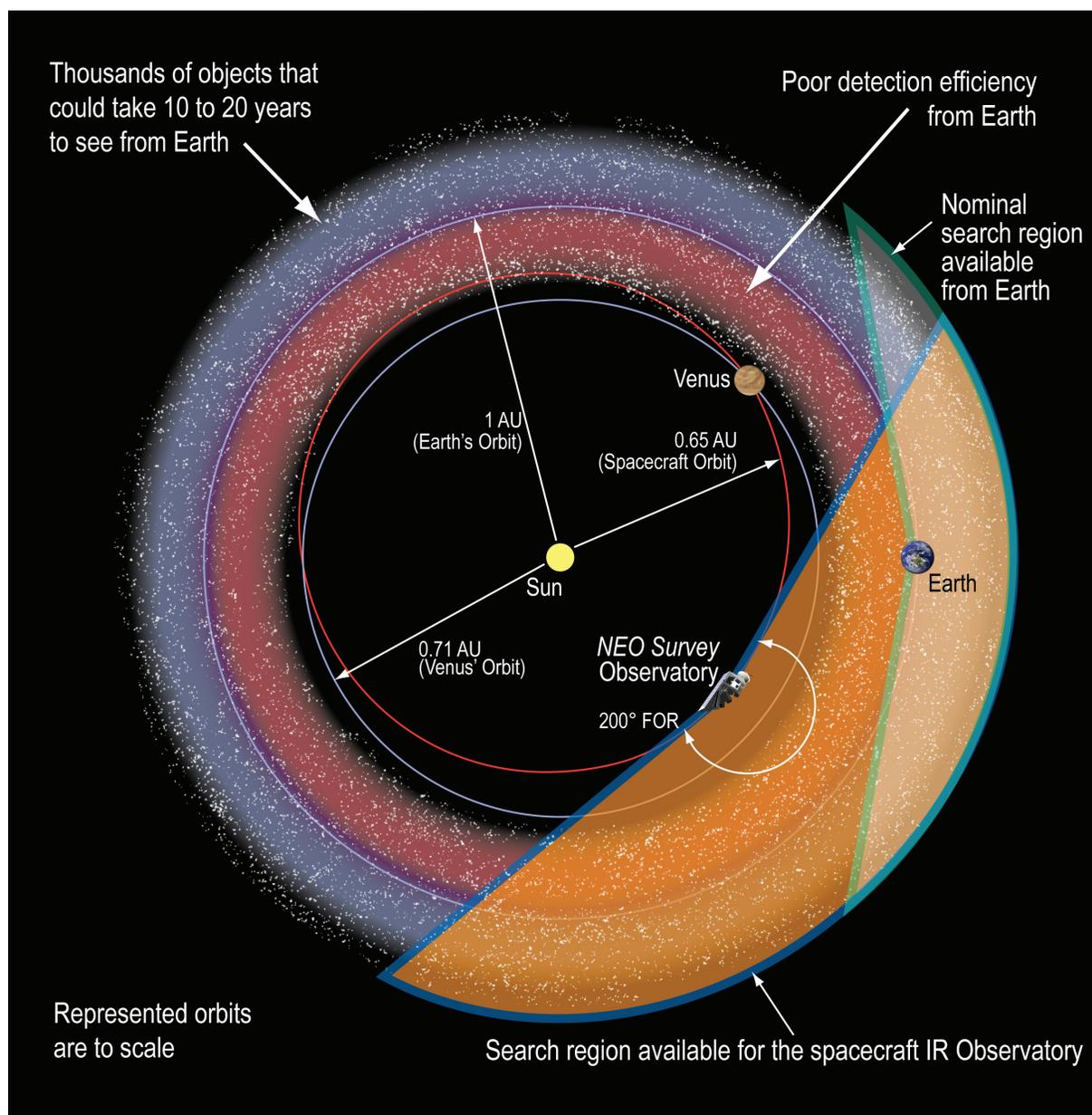
**FIGURE 3.5** The region of the sky observed by the NEO Survey (see text). NOTE: NEO, near-Earth object; AU, astronomical unit; IR, infrared; FOR, field of regard. SOURCE: Courtesy of Ball Aerospace and Technologies Corporation and NASA.
