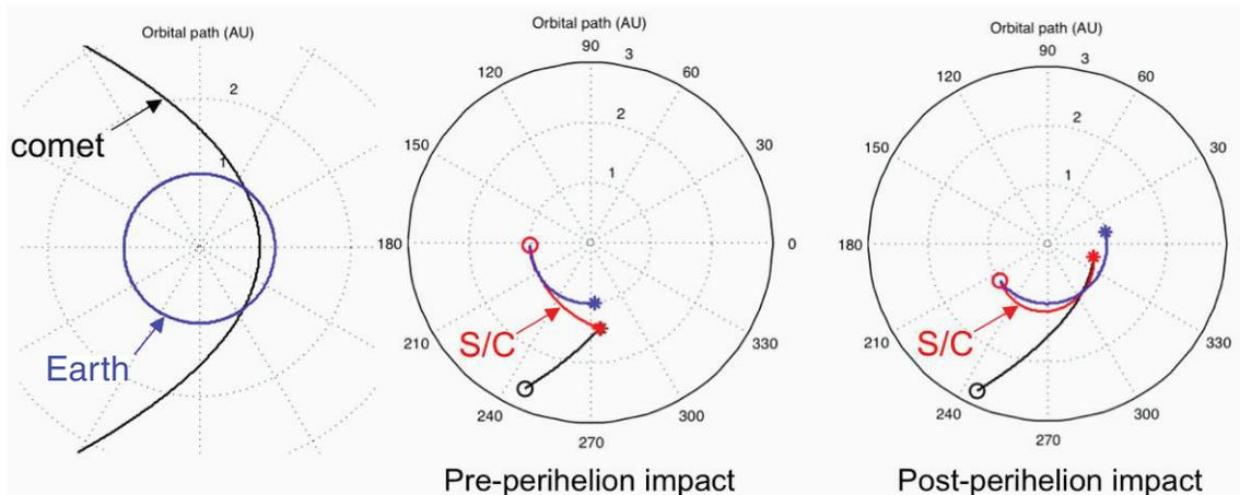
**FIGURE 5.4** Intercept trajectories for a hazardous, long-period comet. The left panel shows the comet's orbit and the two places at which it intercepts Earth's orbit. The next two panels show the intercept trajectories corresponding to the two rows in Table 5.6. In other respects, the panels are similar to those in Figure 5.3.
